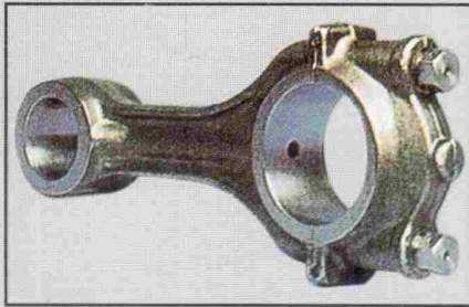
Die forged connecting rod, "split-bolting" type, with rifle drilled oil passage
